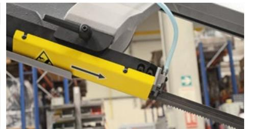
An adjustable guide cube provides the possibility to be set as close to the material as possible.
