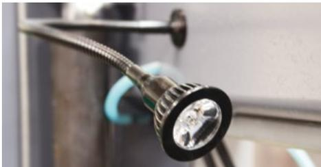
*A LED lamp for lighting the workspace, adjustable and mounted on the flexible arm.*
