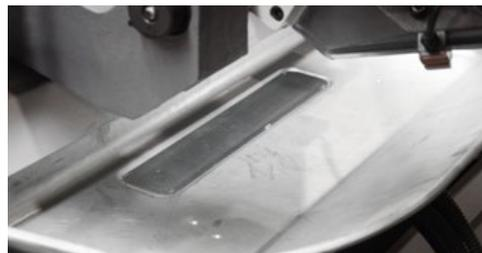
A large, easily accessible chip tray with dripping sieve prevents the coolant from flowing out the machine.
