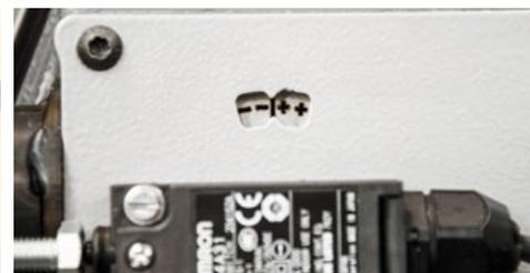
Saw blade tensioning is indicated by a new indicator on the arm.
